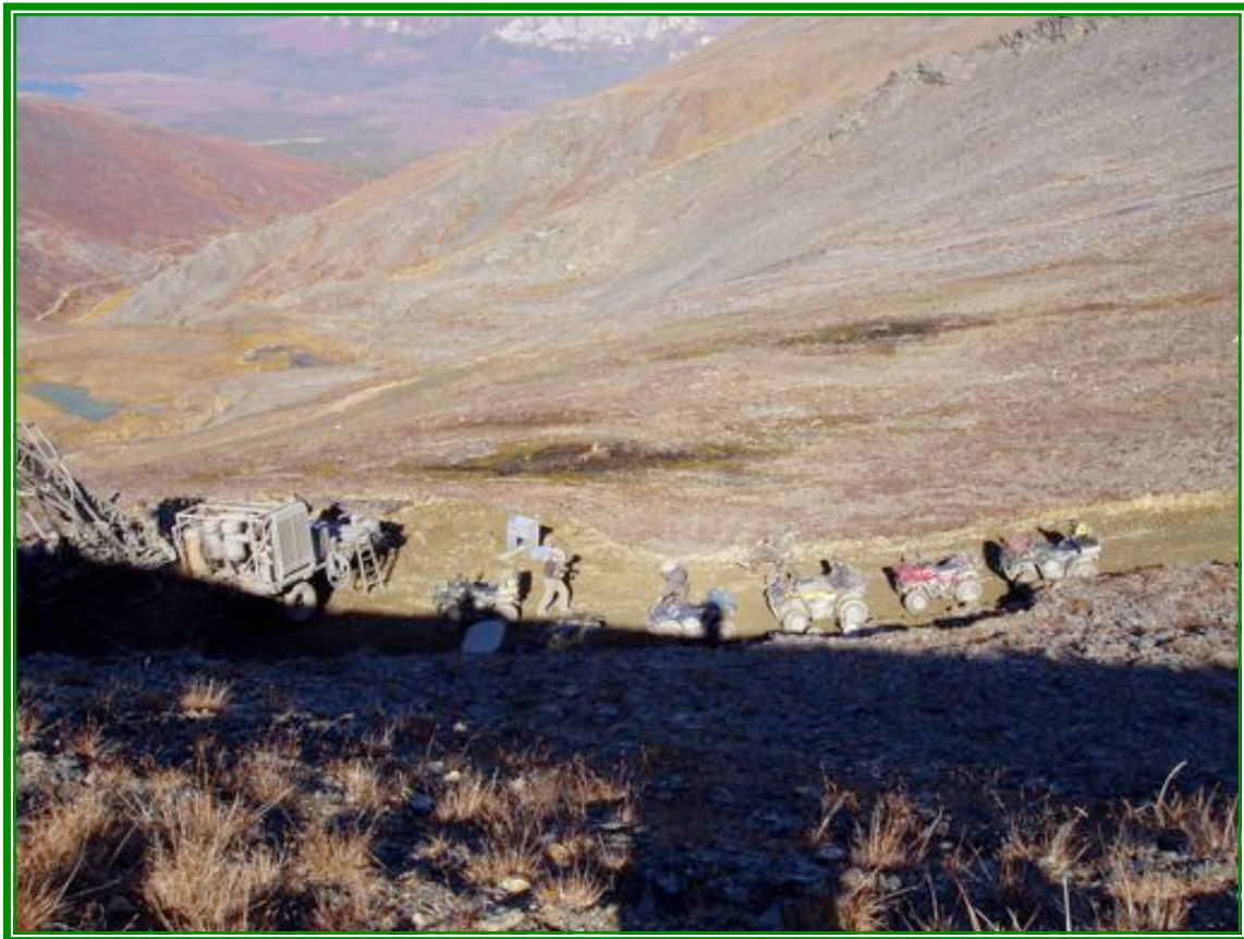
Figure 53. Preparing to drill the Ratchet Ridge prospect. Note the two acidic seep areas and dead vegetation that straddle a quartz vein and directly overlie 1,000-gamma magnetic anomalies later found to be due to magnetic pyrrhotite in auriferous, carbonate altered, mafic rock.
