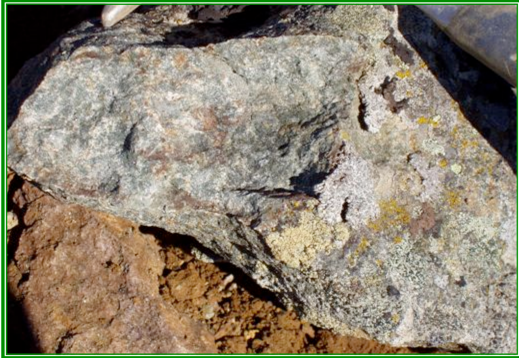
Figure 38. Altered metadiorite(?) with carbonate, sericite, chlorite, Fe-ox, and variable silicification. Carbonate appears to replace plagioclase (sample LS1857).
