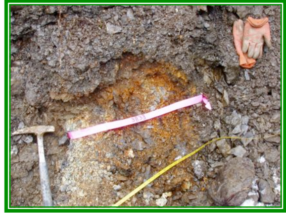
Figure 30a (left). Photograph of trench wall showing location of LS3759, a sample of a 5-inch wide pulverized quartz vein striking 110° in black carbonaceous schist; and Figure 30b (right), a photo of trench channel sample LS3833 from across a two-foot steeply north-dipping and pulverized quartz vein with seams of arsenopyrite.
