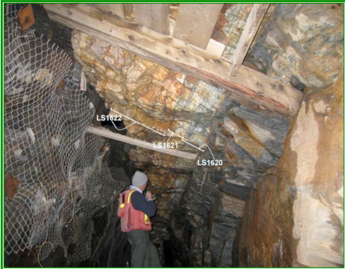
Figure 34. Little Squaw white quartz vein exposed in the 100 Level of the Little Squaw mine. The banded quartz-gold footwall zone (LS1620 and -21) commonly contains 50 or more ppm gold. The view is along strike looking west. Note the open fracture on the hanging wall (between LS1622 and the wire net), likely due to landslide tension resulting from mass downslope transport of sheared rock northeast of the mine site (to the right of photo).
