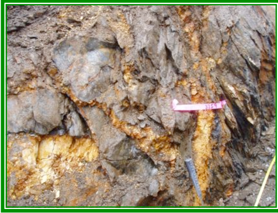
Figure 30a (left). Photograph of trench wall showing location of LS3759, a sample of a 5-inch wide pulverized quartz vein striking 110° in black carbonaceous schist; and Figure 30b (right), a photo of trench channel sample LS3833 from across a two-foot steeply north-dipping and pulverized quartz vein with seams of arsenopyrite.
