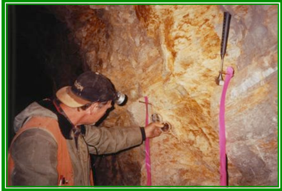
Figure 35a (left): Example of an 8-foot wide siderite-carbonate altered NW fault zone, with a 58° northerly(?) dip showing left lateral movement as seen on the 200 Level cross-cut; within this fault zone are north-dipping NE slickenside and shallow north-dipping faults with cm-scale, right-lateral displacement. Figure 35b (right): normal dip-slip movement on a NW-striking fault dipping 45° NE.
