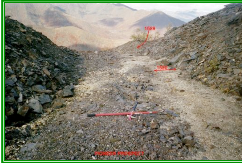
Figure 50 - 1981 dozer trench showing pinching and swelling auriferous quartz lenses.
