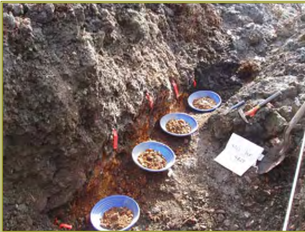
Figure 20. Trench sample collection technique; each interval is divided into quadrants, equal amounts of sample are cut from each quadrant, then composited into the interval sample.
