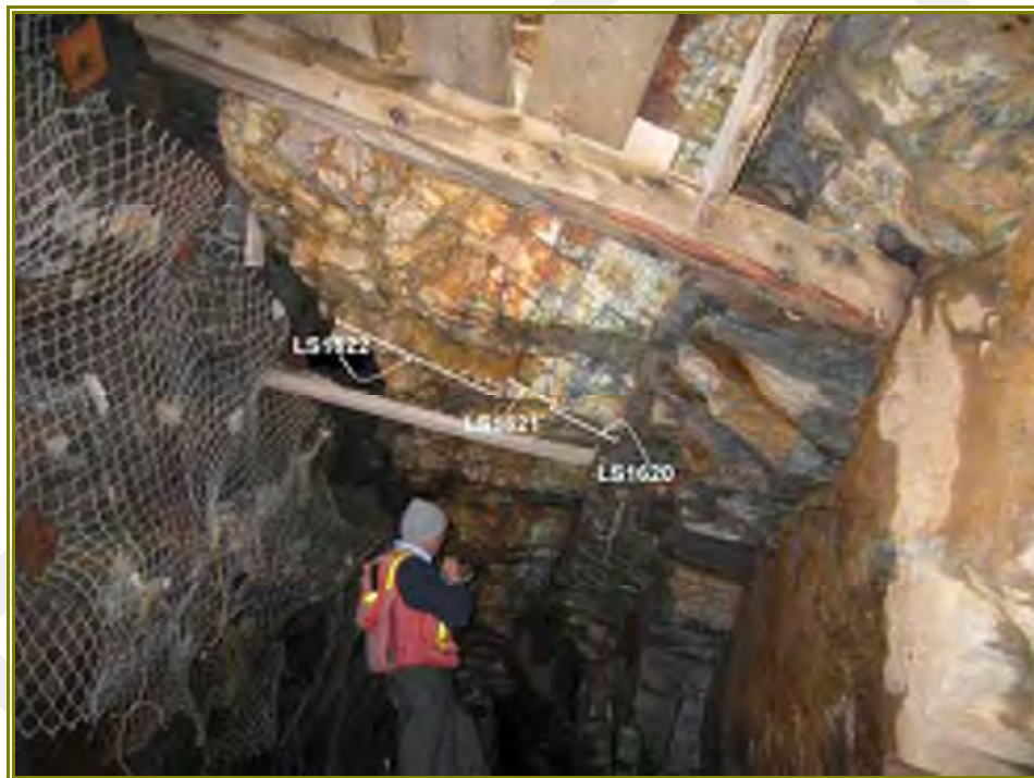
Figure 16. Looking west along the 100-Level ore shoot of Little Squaw quartz vein, a banded quartz-gold footwall zone.
