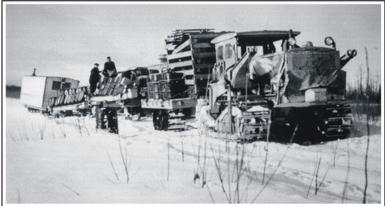
Figure 25. A typical cat-train in the late 1930s, delivering fuel to a mining camp during winter. The wanagan at the rear of the train was the crew quarters during the trip. This cat-train was traveling from Aniak to Flat. Eddie Barge collection, OHA/BLM Flat Project, OHA, Anchorage.
