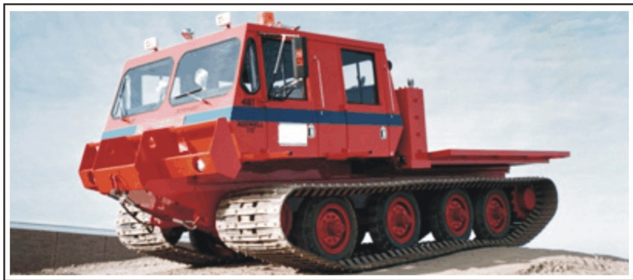
Figure 56. A Nodwell 110 tracked vehicle, similar to those used for hauling freight on the Coldfoot-Chandalar Trail and for oil exploration on the North Slope. Photo courtesy of Formost Industries LP.
