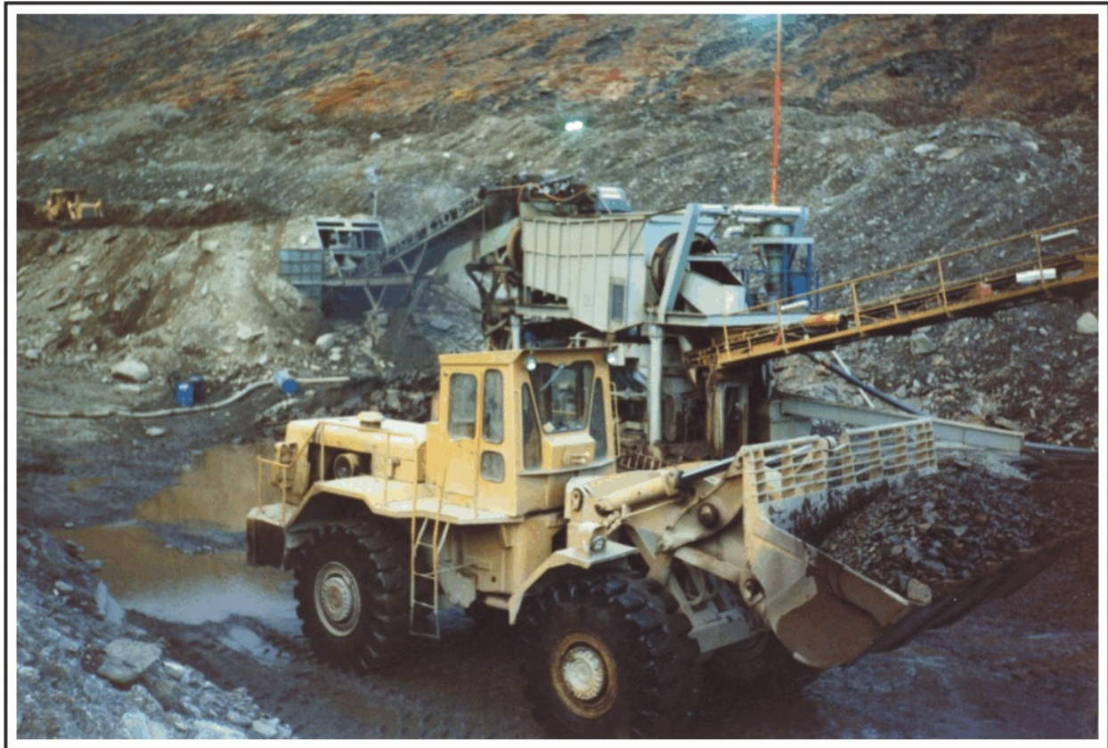
Figure 53. Del Ackels' dry-land jig recovery plant at his placer mine on Tobin Creek, 1991. Eskil Anderson Collection, courtesy of Richard Walters, LSGMC, Spokane.
