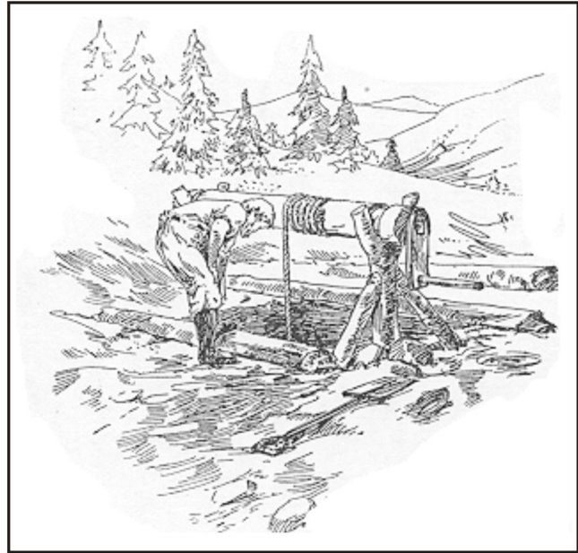
Figure 6. A drift mine windlass. Drawing from the University of Alaska Archives, Consortium Library, Anchorage.
