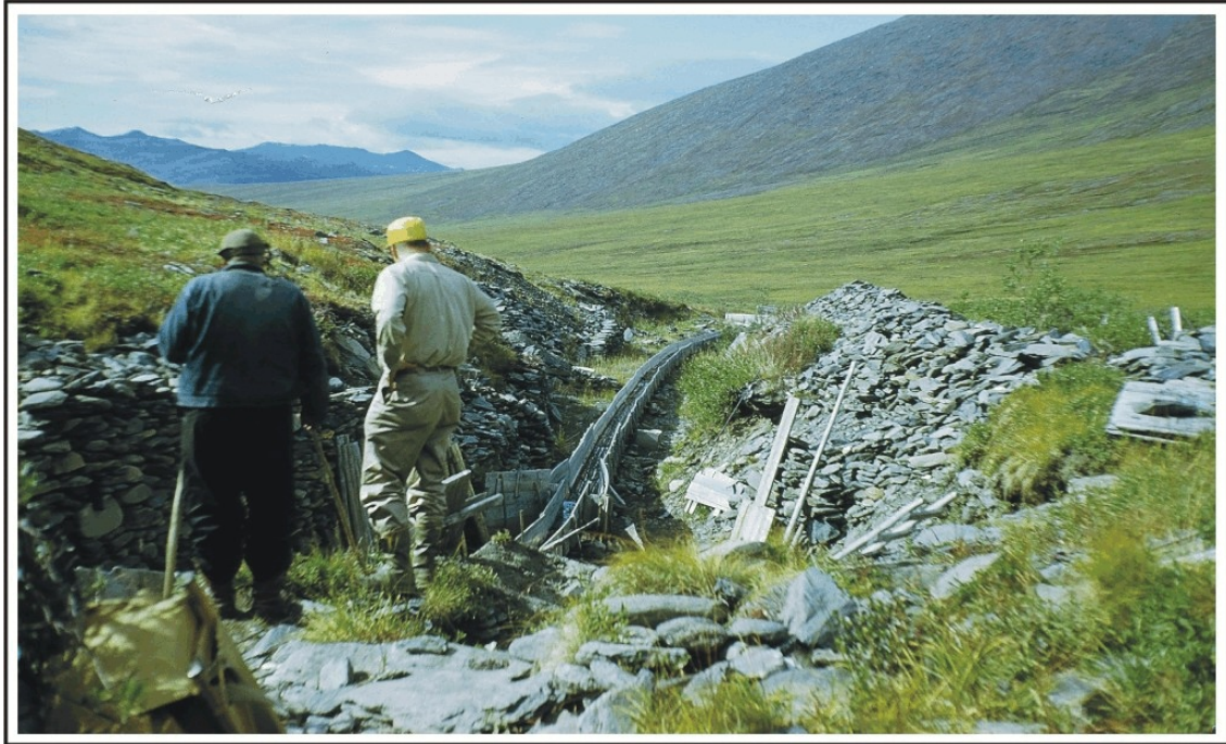
Figure 32. Ellis Anderson (left) and Eskil Anderson (center) at the former's sluice boxes on a bench on Tobin Creek, 1957. Eskil Anderson Photo Collection, courtesy of Richard Walters, Spokane, Washington.
