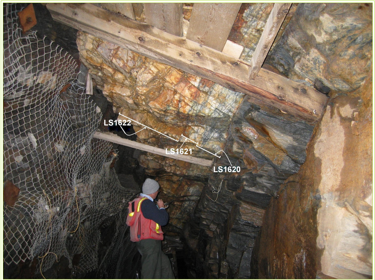
Figure 13. Massive white quartz (left), including a banded quartz-gold footwall zone (right) of the Little Squaw vein, is exposed at the 100 Level of the Little Squaw Mine. The banded zone contains multiple oz gold per ton. The vein is about 4 feet thick at this location and the view is along strike looking west. Note the open fracture on the hanging wall, likely due to landslide tension resulting from mass downslope transport of ground to the northeast of the mine site.
