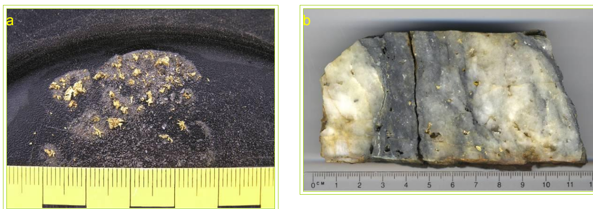
Figure 6. Nugget effect: a) Fragments of gold shed from vein-quartz ore shoot debris of the Little Squaw vein and recovered by a gold pan; b) gold-bearing quartz from the site of LS1620, which assayed 89.2 oz. Au/ton over 9 inches, the adjoining 7-inch channel sample assayed only 60 ppb. Visible gold grains are up to 3 mm in size in both photos.
