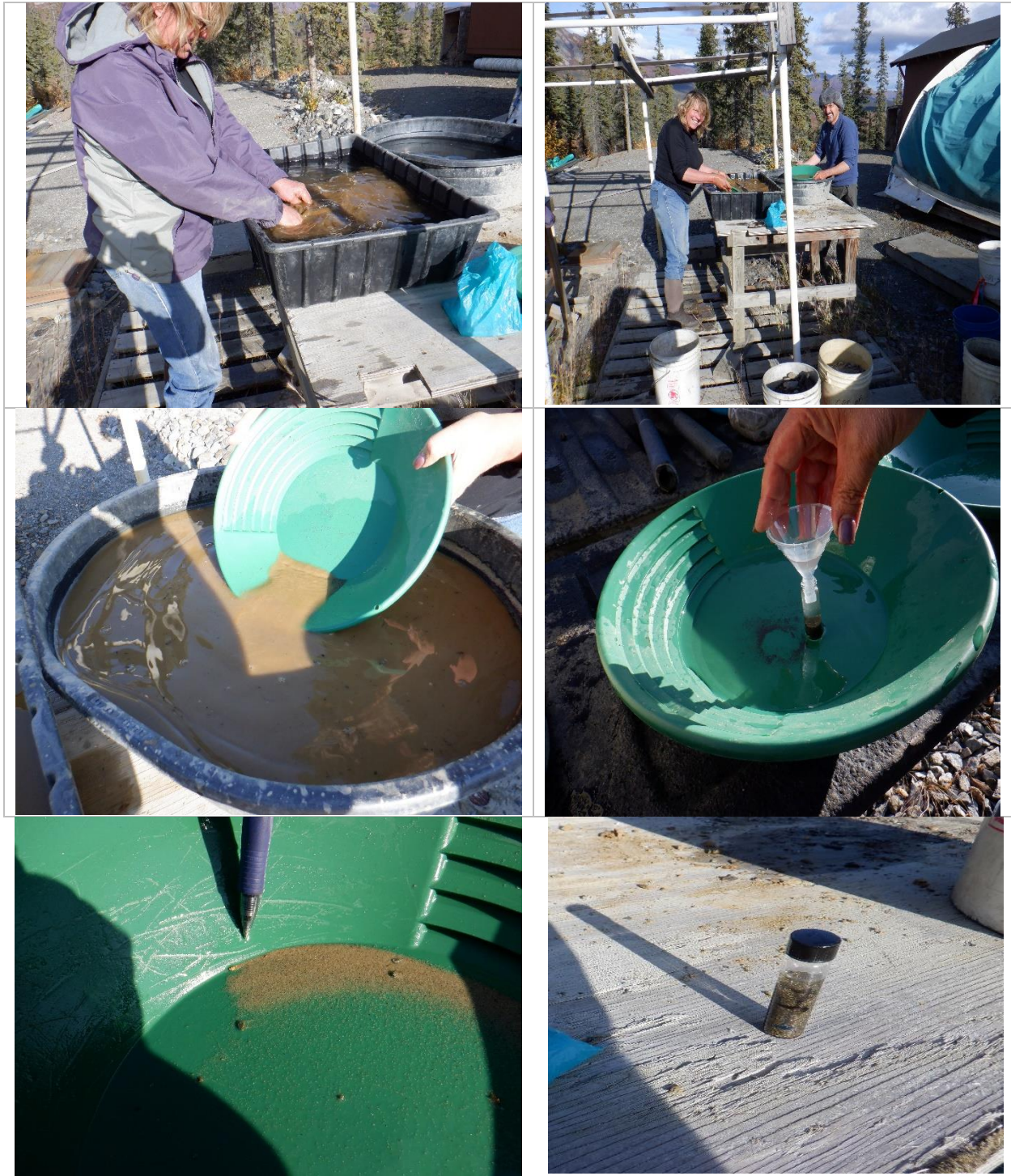
Photo 12-3: GRE Panning at the Chandalar Mine and Collecting the Fine Size in the Vial
